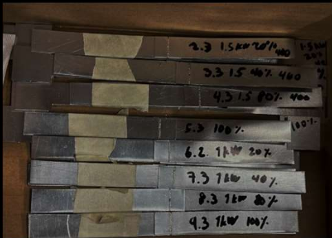
Al-Al welds for battery applications Example: Al busbar + Al Casing for cells (Bachelor thesis)
