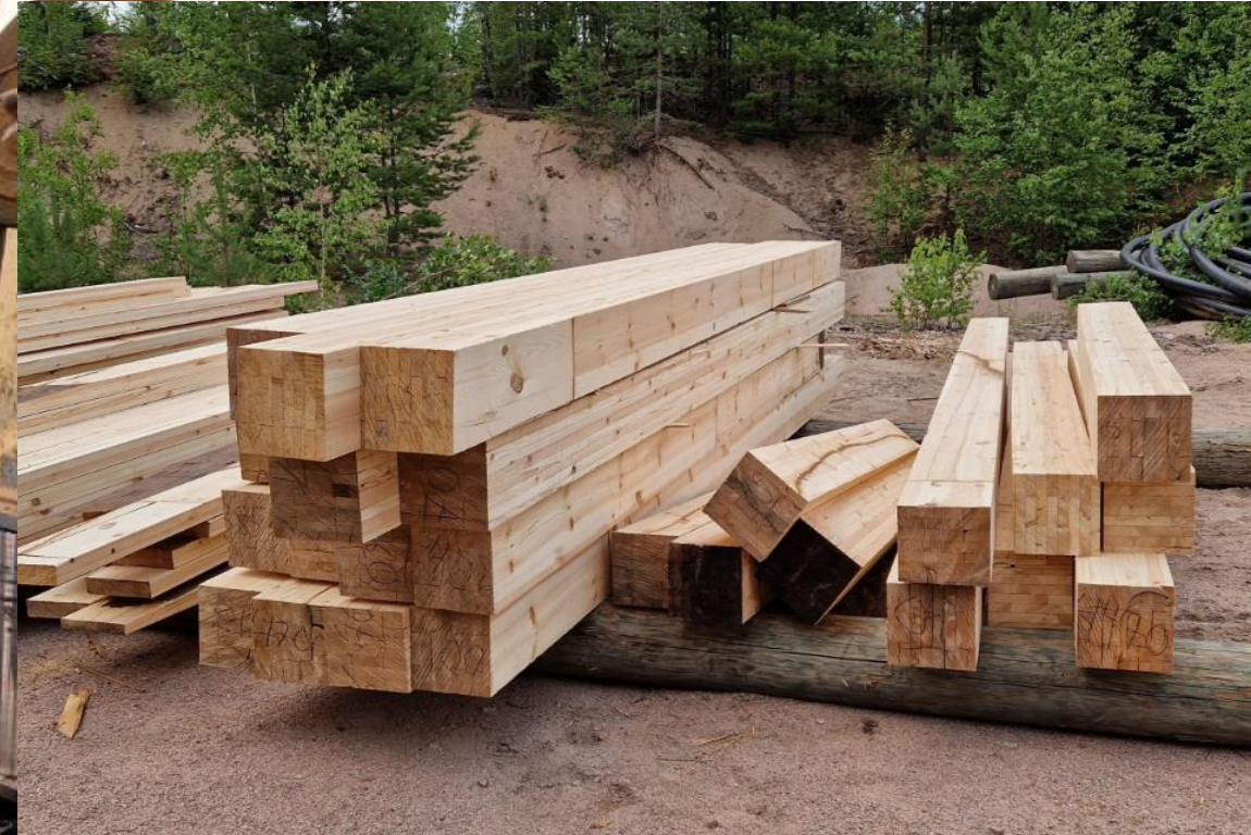
Collecting and refining the chosen materials: Sawn off glulam timber structures ready for the transportation to Messukeskus.
