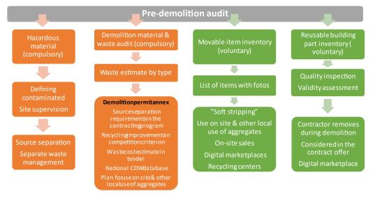
Figure 15. Components and outputs of the pre-demolition audits (figure Raimo Lilja and Jenina Luotolampi)
