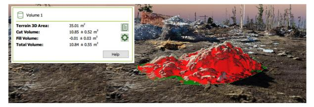
Figure 4 Volume calculation from a material pile based on drone imaging and 3D modelling (figure Juha Vihavainen).
