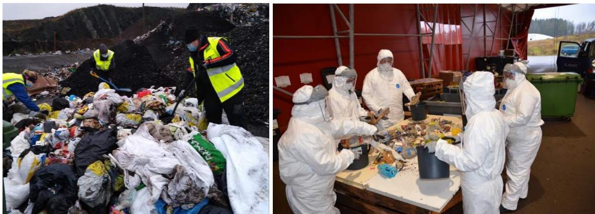
Figure 8. Composition study was performed to find out the share of recyclable bio-waste in household mixed waste of Peitsari area before and after demonstration actions. Left: sampling. Right: manual sorting of mixed waste. (Photos Hanne Soininen and Anne Laitinen).
