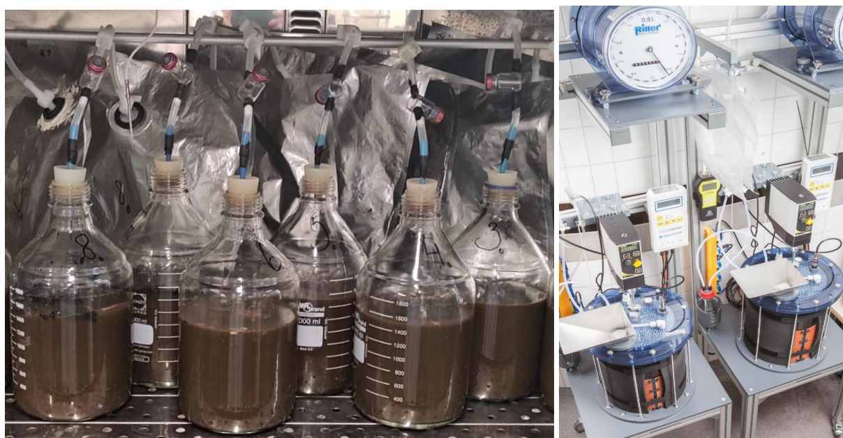
Figure 13. 2 L bottle batch reactors and 15 L pilot scale reactors were used in the demonstration experiments to optimize dry fermentation process of bio-waste (photos Tiina Saario (left) and Manu Eloaho (right)).
