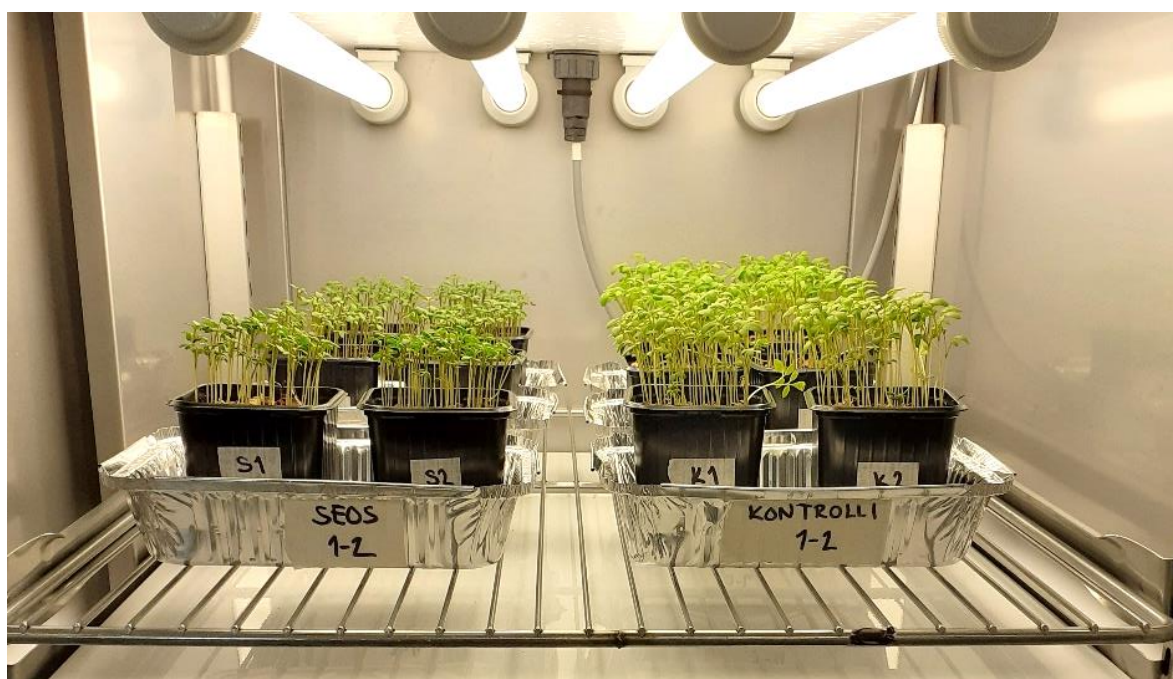
Figure 18. Plant growth tests were performed for soil improvement product and pelletized granules produced from bio-waste-based digestate of biogas plant (photo Janne Junninen).
