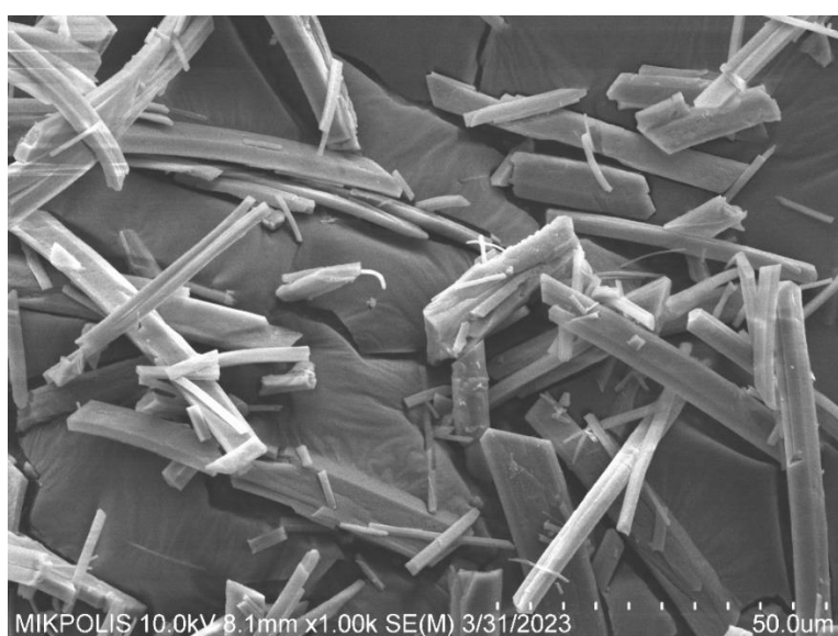
Figure 16. A scanning electron microscope (SEM) picture from struvite precipitate recovered with electrochemical method from liquid fraction of biowaste digestate. (Picture Xamk, Mikpolis laboratory)
